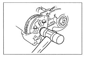
14. Tap in the new blind cap by using a plastic hammer.
